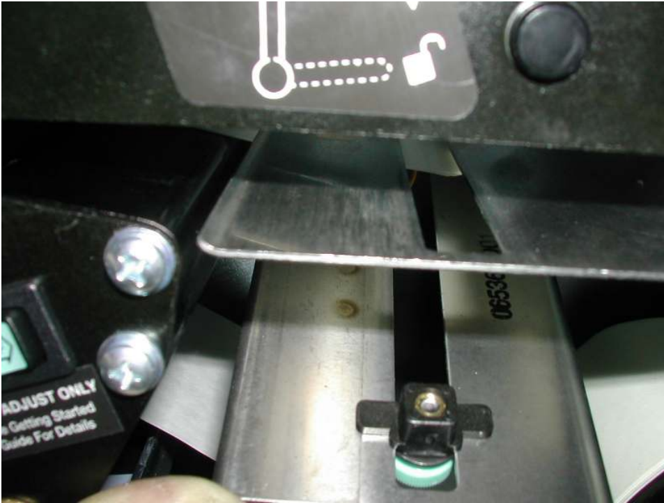
Label edge guide assembly installed in lower media guide.
